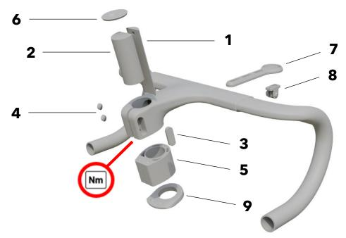
! Maximum torque of cockpit bolts: 6 Nm
