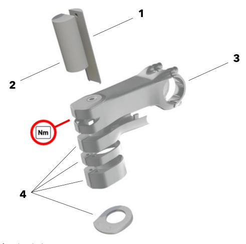
! Maximum torque of cockpit bolts: 6 Nm
