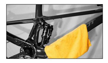
4. Loosen and remove the lower shock bolt.
