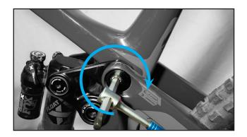
3. Remove the flip chips from both sides. Pushing on the bolt from inside the link can make it easier to get the chips out. The form of the chip only allows it to go in to the oval pocket two ways.
