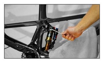
29. Use a towel or rag to wipe any excess Loctite from mounting locations. Loctite can damage paints and finishes.
