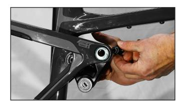
21. Torque both flip chip bolts to 35 Nm.
