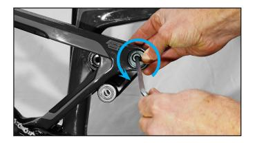
22. Apply a small amount of Loctite 243, or equivalent, to the lower shock frame threads. Spread evening with a wooden toothpick. Loctite can damage paints and finishes so use caution.
