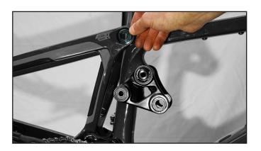
14. Grease the frame contacting surfaces of the flip chip or the flip chip pocket on the frame. Take care not to get any grease on the threads.
