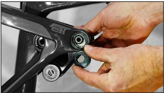
9. Carefully rotate the lower link forward out of the rear triangle to not drop the washers.
