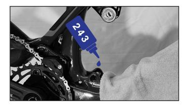
19. Insert one of the flip chip bolts through the link and frame and align with the flip chip.
