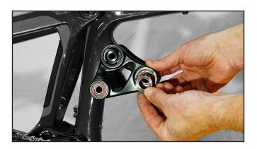
11. With the chips, bolts, and washers removed clean any residual grease and threadlocker off the surfaces of all the parts. Isopropyl alcohol is recommended to clean all the parts before reassembly.
