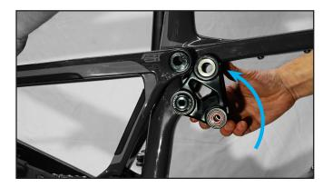
20. Use a 6mm wrench to snug the bolt into the flip chip. Repeat this process on the other side.
