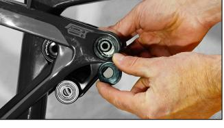
8. Loosen and remove the flip chip bolts.
