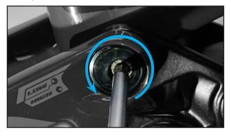
3. Align and install the flip chip on the other side of the bike.
