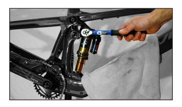
25. Apply Motorex Bike Grease, or equivalent, to the head and shaft of the bolt, but not on the threads.
