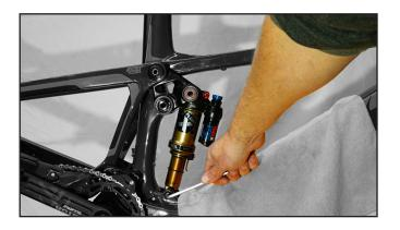
27. Torque trunnion bolts and lower shock bolt to 13 Nm.
