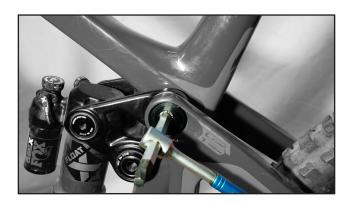
4. Torque both flip chip bolts to 35Nm.
