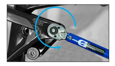
23. Apply a small amount of Loctite 243, or equivalent, to the trunnion mount threads. Spread evenly with a wooden toothpick.
