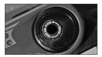
2. Begin by loosening the flip chip bolts using a 6mm hex wrench. The bolts are inserted from the inside of the link so to loosen them from the outside you will need to rotate the wrench clockwise.
