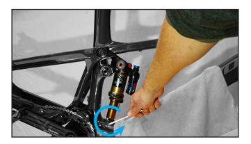
6. Lift the rear triangle to rotate the upper link to access the flip chip bolts from the inside.
