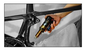
2. Place a towel or rag on the downtube to protect it when removing the shock.
