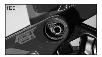
2. Align the flip chip with the bolt and begin threading it in by rotating the bolt counter-clockwise. Check that the flip chip is properly aligned in the frame for your chosen riding position. *Do not tighten completely until you have aligned the flip chip on the other side of the bike.*
