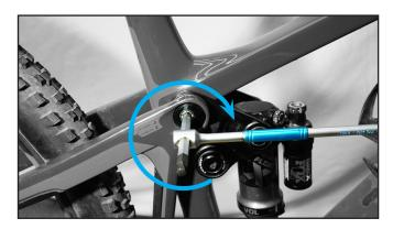
3. Loosen and remove the two trunnion mounting bolts from the upper link.
